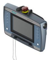
SIMATIC HMI KTP700F Mobile Arctic, (extended operating temperature range), 7.0" TFT display, 800x 480 pixel, 16m colors, key and touch operation, 8 function keys, 1x PROFINET/Industrial Ethernet interface, 1x multimedia card, 1x USB, 1x touch pen, keyswitch, acknowledgement button, emergency shutdown/stop button, configurable from WinCC Comfort V15 SP1
