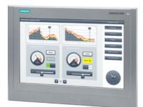
SIMATIC HMI TP1500 Comfort Outdoor, Comfort Panel, Touch operation, 15" widescreen TFT display, 16 million colors, PROFINET interface, MPI/PROFIBUS DP interface, 12 MB configuration memory, Windows CE 6.0 (Microsoft Support included Security updates discontinued) configurable from WinCC Comfort V13 SP1, HSP
