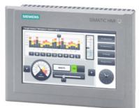
SIMATIC HMI TP700 Comfort Outdoor, Comfort Panel, touch operation, 7" widescreen TFT display, 16 million colors, PROFINET interface, MPI/PROFIBUS DP interface, 12 MB configuration memory, Windows CE 6.0 (Microsoft support including security updates discontinued) configurable from WinCC Comfort V13 SP1, HSP
