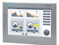
SIPLUS HMI TP1500 Comfort Outdoor based on 6AV2124-0QC13-0AX0 with conformal coating, -30...+60 °C, TP1500 Comfort Outdoor, Comfort Panel, touch operation, 15" widescreen TFT display, 16 million colors, PROFINET interface, MPI/PROFIBUS DP interface, 12 MB configuration memory, Windows CE 6.0, configurable WinCC Comfort V13 SP1 and higher, HSP
